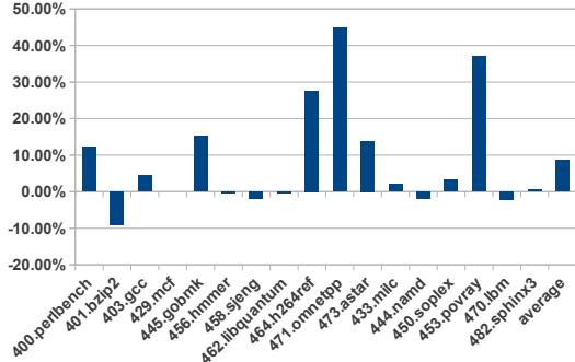
Figure 11: SPEC CPU2006 Benchmark Performance
