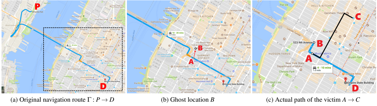
Figure 3: An attack example: the victim’s original navigation route is P \rightarrow D ; At location A, the spoofer sets the GPS to a ghost location B which forces the navigation system to generate a new route B \rightarrow D . Following the turn-by-turn navigation, the victim actually travels from A to C in the physical world.
